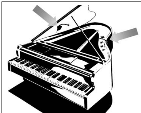
Fig. 9: Miking up a grand piano with two C 516 MLs
