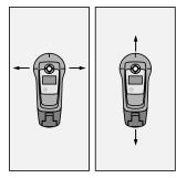
In order to achieve best results, the tool should be used with a sweeping motion (extended horizontal and vertical, back and forward movements over the object). The series of illustrations shows the sweep scan technique in use.
