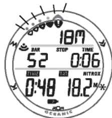
Fig. 100 - DELAYED VIOLATION #2 MAIN
