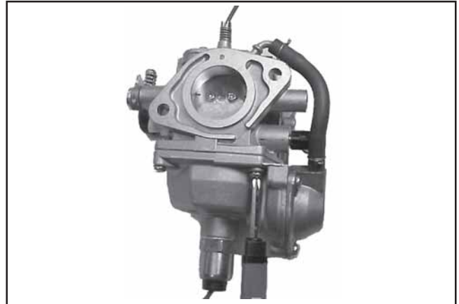
Figure 5-13. Installation de la cuve de carburant.
