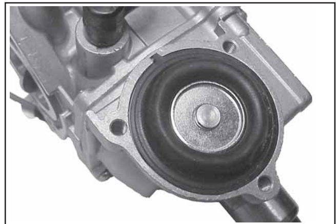
Figure 5-30. Membrane en place.
