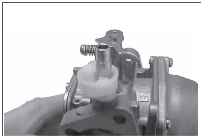
Figure 5-34. Installation du coussinet.
