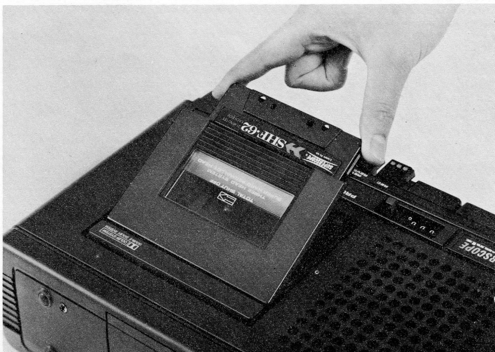
Figure 4. Installation de la Cassette
