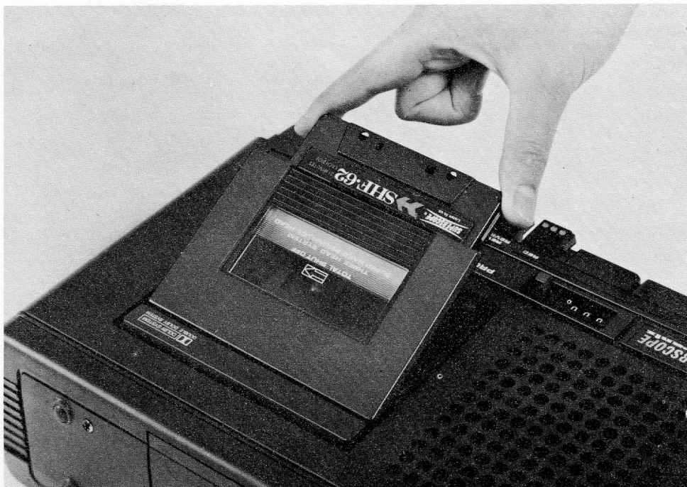
Figure 4. Installation de la Cassette
