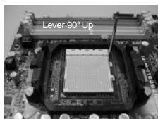
STEP 1: Lift Up The Socket Lever
