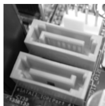
eSATAII connectors (eSATAII_TOP (Port4) and eSATAII_BOTTOM (Port5))
