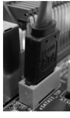
Connect the SATA data cable to the eSATAII connector (eSATAII_TOP)
