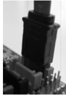
Connect the SATA data cable to the red SATAII connector (SATAII_RED (PORT 1))
