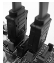
Connect the SATA data cables to both red SATAII connector (SATAII_RED (PORT1)) and orange SATAII connector (SATAII_ORANGE (PORT3))
