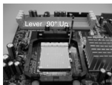
STEP 1: Lift Up The Socket Lever
