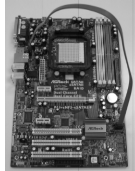
Connect the SATA data cable to the red eSATAII connector (eSATAII_BOTTOM)
