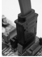
Connect the SATA data cable to the red SATAII connector (SATAII_RED (PORT1))
