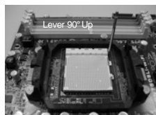
STEP 1: Lift Up The Socket Lever
