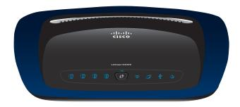
1, 2, 3, 4 (Green/Blue) These numbered LEDs, corresponding with the numbered ports on the Router's back panel, serve two purposes. The LED is continuously lit when the Router is connected to a device through that port. It flashes to indicate network activity over that port. The LED lights up green when the port is connected to a gigabit port or blue when the port is connected to a 10/100 port.
