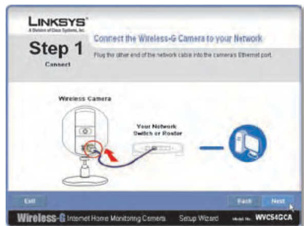
Connect Network Cable to the Camera
