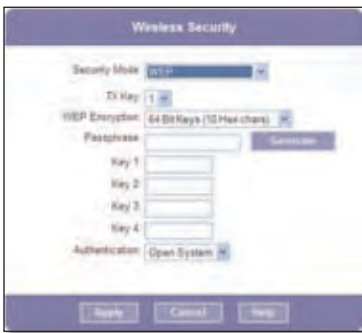
Wireless Security, WEP: WLAN-beveiliging ingeschakeld in WEP-modus
