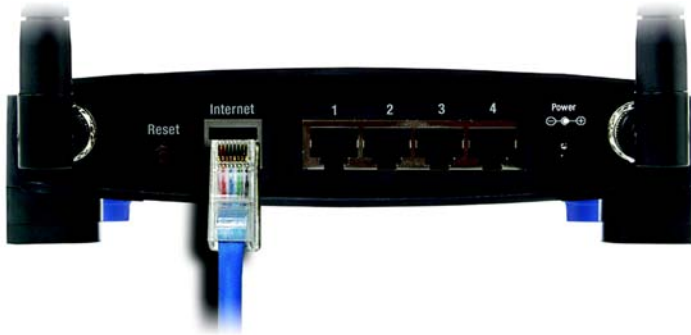
Figure 4-6: Connect the Broadband Router's Internet Port to the other Router's Numbered Ethernet Port
