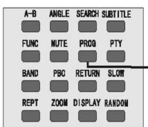
1. Make sure that there is a data carrier in the device. Press the PROG button to display the programming table on the screen:
