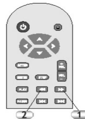
1. Press the right side of the button to search in fast forward. Press the button repeatedly to search at different speeds.
