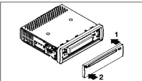
First place the operating panel in position on the right-hand side and then lock it into place on the left.
