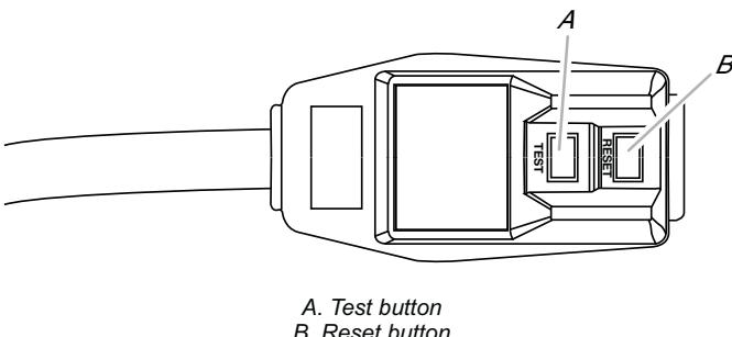
This room air conditioner is equipped with a power supply cord required by UL. This power supply cord contains state-of-the-art electronics that sense leakage current. If the cord is crushed, the electronics detect leakage current and power will be disconnected in a fraction of a second.
