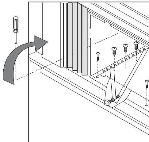
5. Use a wood block between the leveling bolts and the wall if the wall is weak or if the weight of the air conditioner falls between the studs in the wall.
