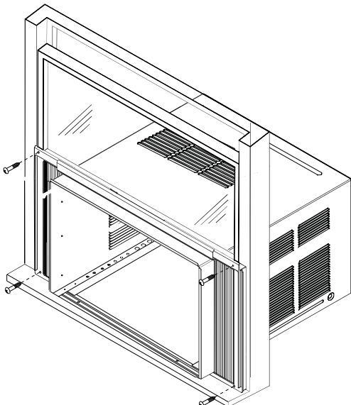
**NOTE: To make screws easier to drive, drill a pilot hole into the sash through clearance hole in curtains.**
