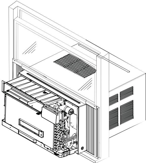
**CAUTION:** For security purposes, reinstall screws at cabinet's sides, removed in step one.
