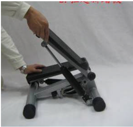
1. Hook the Cable on the wheel.
