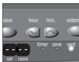
L: A blinking VENT indicator light is a sign that you need extra ventilation.
