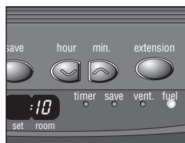
K: When the FUEL indicator light is lit, the information display will show the number of minutes of fuel left in the tank.
