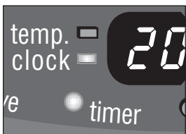
H: The TIMER indicator light indicates that the timer function has been switched on.
