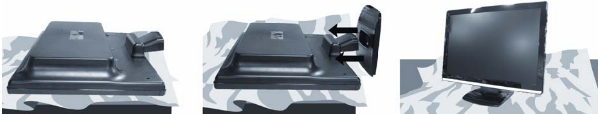
(III.: Installation of the monitor stand)
