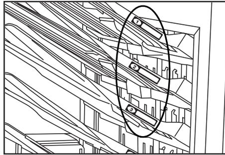
\* Attach the seals in the location indicated in the illustration. The locations to which seals are applied are ①, ②, ③, ④, and ⑤ from the top.
