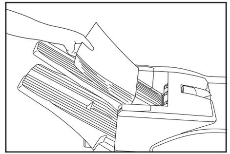
\* If the Stacking mode does not engage and the number of finished copies in the Tray (B) reaches the acceptable limit, an error message will be displayed on the copier and copying will stop. Remove all of the finished copies from the Tray (B) and then resume copying.
