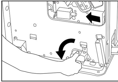
2. Turn the Unit release lever, and hold the Unit release handle to move the Center-folding unit in the paper ejection direction.
