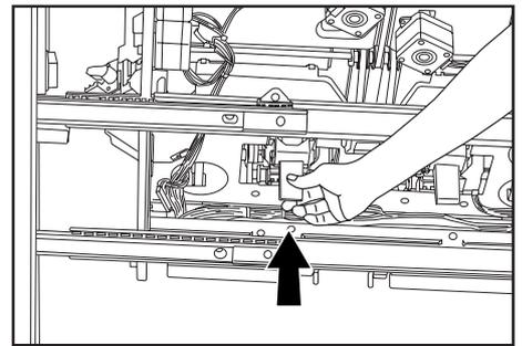
7. Replace the staple holder back in its original position in the stapling unit. Once it has been fully inserted, it will click into place.
