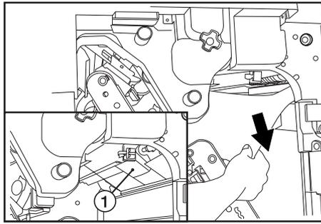
5. Hold the Coupling section guide lever ① and open the Coupling section guide.
