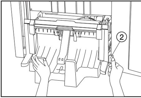
7. Close the Conveyor guide and push in the Center-folding unit to its original position while pressing the Center-folding unit installation button ②.
