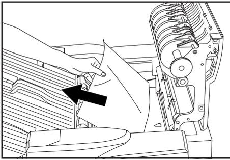
2. Open the Upper cover and remove the jammed paper.
