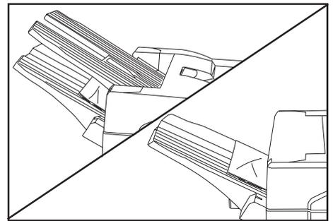
\* Copies will be ejected to Tray (A) in the single-staple mode and to Tray (B) in the Double-staple model. If the bypass is used, copies will be ejected to Tray (A).
