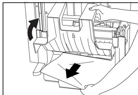
6. Open the Storage cover upward and remove any jammed paper. If the paper is removed, lower the Storage cover.
