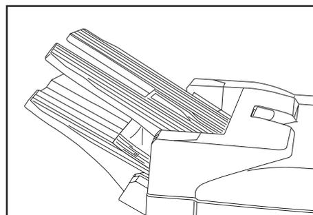
4. Press the Start key. The copies will be automatically stapled and ejected onto the Tray (A).
