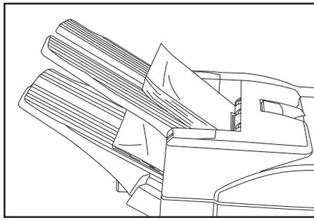
\* If the number of copies exceeds the capacity of Tray (B), the stacking mode will be activated and copies will be ejected to Tray (A).
