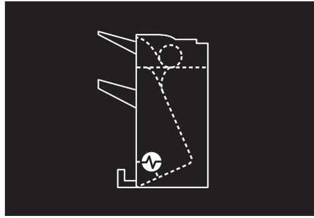
● **Paper jam in the ejection section of optional Center-folding unit**
