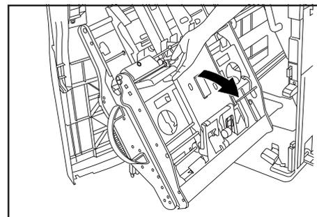
5. Hold the Internal tray release lever and open the Internal tray.
