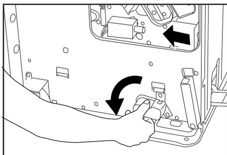
2. Turn the Unit release lever, and hold the Unit release handle to move the Center-folding unit in the paper ejection direction.
