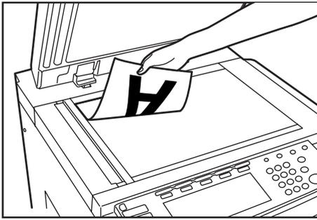
\* When setting an original on the platen, a message will appear after each original is scanned to confirm whether you want to scan another original or not. Refer to the Operation Guide of your copier for further details.
