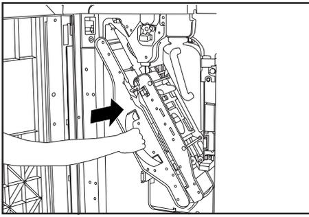
8. Replace the internal tray in its original position all the way into the Finisher.
