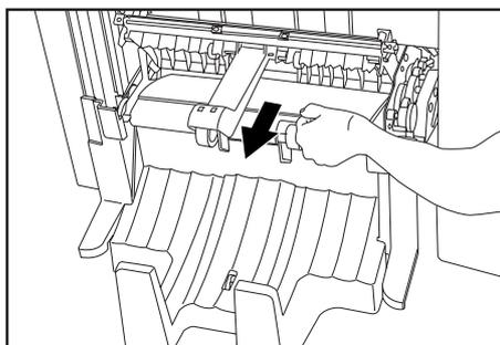
5. Hold the Conveyor guide lever to open the conveyor guide and remove the jammed paper.
