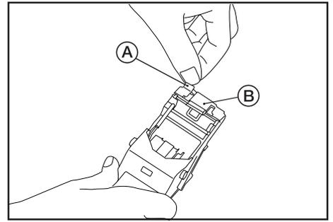
4. Push the knob (A) of the face plate of the staple holder to open the cover plate (B).
