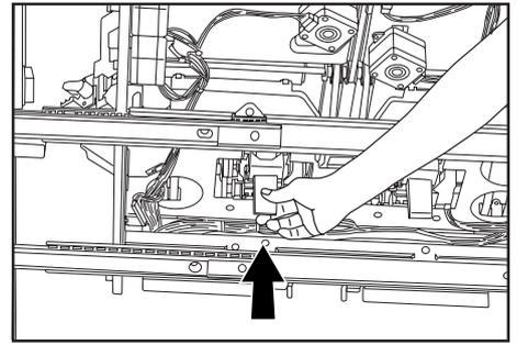
8. Replace the staple holder back in its original position in the stapling unit. Once it has been fully inserted, it will click into place.
