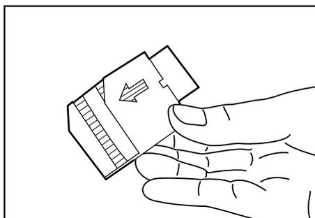
5. Remove the new staple cartridge from its box.
