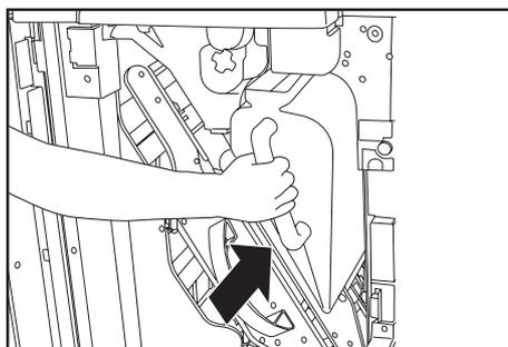
4. Insert the Scrap hole-punch box by aligning it with the guide of the finisher.
