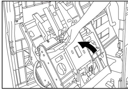
7. Hold the Internal tray release lever and close the Internal tray.
