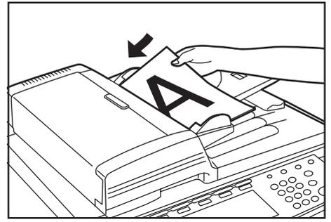
6. Reset the previous original(s) and press the Start key. The copy job that was interrupted will then resume.
