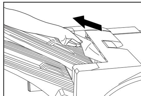
1. If the jammed paper is visible in the eject slot, pull it out in the direction shown in the illustration without tearing it. If the jammed paper cannot be removed, proceed to the next step.
