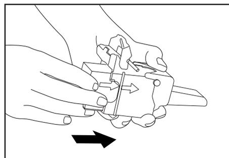
6. Hold the staple holder in one hand and the new staple cartridge in the other and insert the new staple cartridge making sure the direction of insertion is correct.
