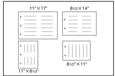
\* The copy paper sizes that are acceptable for hole-punching and the available positioning and number of holes differs depending on the specifications for your unit.
