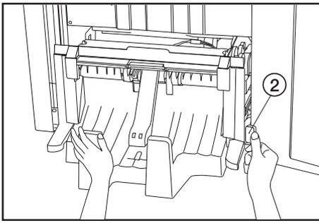
5. Close the conveyor guide and push in the Center-folding unit to its original position while pressing the Center-folding unit installation button ②.
