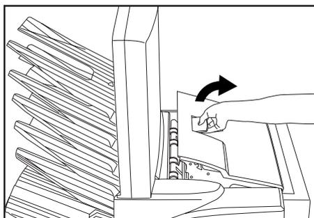
2. If the paper is not easy to remove, open the Upper cover of the finisher and remove the jammed paper. (Refer to page 64.)
