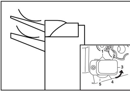
3. If ejected copies are curling upward in a mode in which sorting is not performed, turn the nip roller adjusting knob in the direction that decreases the number indicated at the hole.
