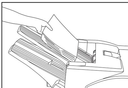
4. Press the Start key. The copies will be automatically hole punched and ejected onto the Tray (B).
