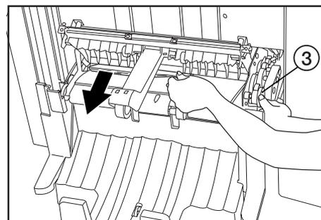
4. If the paper is not easy to remove, turn the Conveyor guide knob ③ to feed the paper to a location where the paper can be easily removed, and remove the paper.
