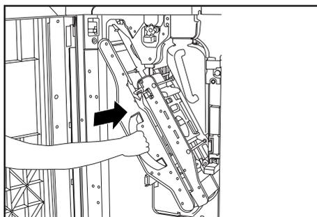
9. Replace the internal tray in its original position all the way into the Finisher.
