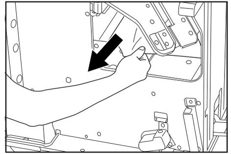
3. If paper is seen from under the Internal tray, remove the jammed paper.
