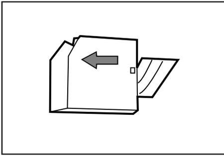
\* The arrow on the staple cartridge indicates the correct direction of insertion.
