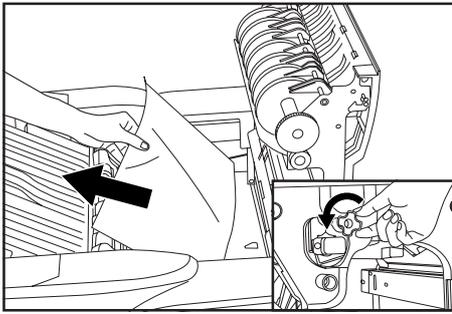
3. Turn the conveyor knob to feed the paper to a location where the paper can be easily removed, and remove the paper.
