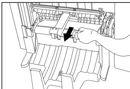
3. Hold the conveyor guide lever to open the Conveyor guide and remove the jammed paper.
