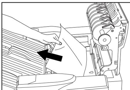
1. Open the Upper cover and remove the jammed paper.
