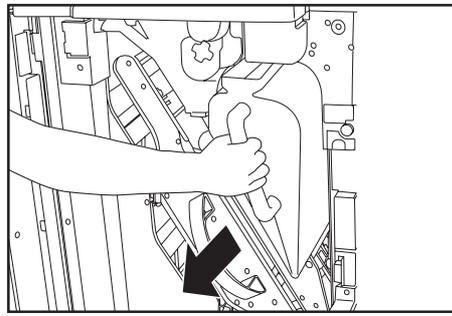
2. Grasp the scrap hole-punch box handle and remove the box from the Finisher.
