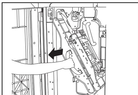
4. If a paper jam occurs in the Internal tray, hold the Internal tray handle and gently pull out the Internal tray toward you. Remove the paper jammed in the Internal tray.
