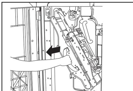
4. Grasp the internal tray handle and carefully pull the internal tray out towards you.
