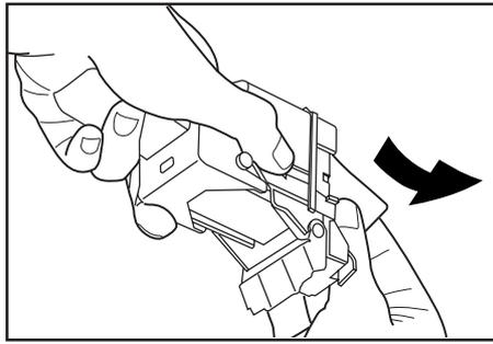
7. Make sure the new staple cartridge is completely inserted all the way into the staple holder and then remove the paper tape covering the staple cartridge.
