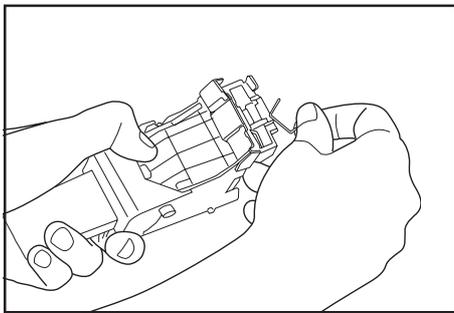
5. Remove the jammed staple from the tip of the staple cartridge (the end where staples are set).
