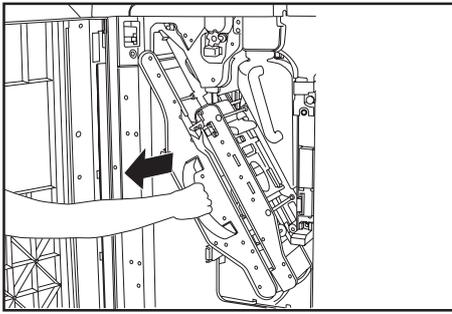
2. Grasp the internal tray handle and carefully pull the internal tray out towards you.
