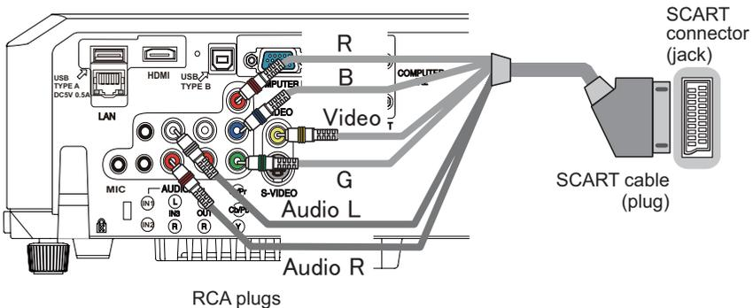
To input SCART RGB signal to the projector, use a SCART to RCA cable.
