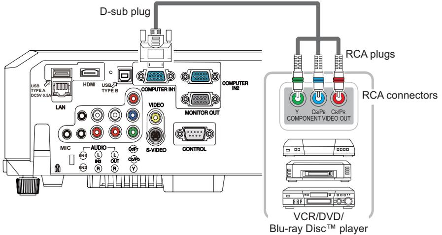
To input component video signal to the **COMPUTER IN1** or **IN2** port of the projector, use a RCA to D-sub cable or adapter.
