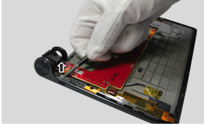
Figure 8-4 Removing the USB FPC holder
