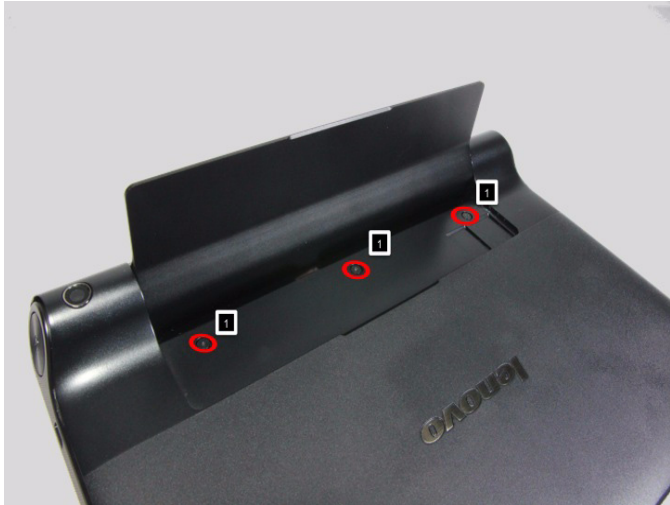
Figure 1-2. Screws on the rear cover
