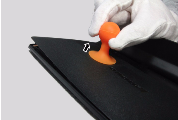
Figure 1-4 Unlocking the central area of the rear cover
