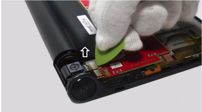
Figure 3-1 Disconnecting the main FPC
