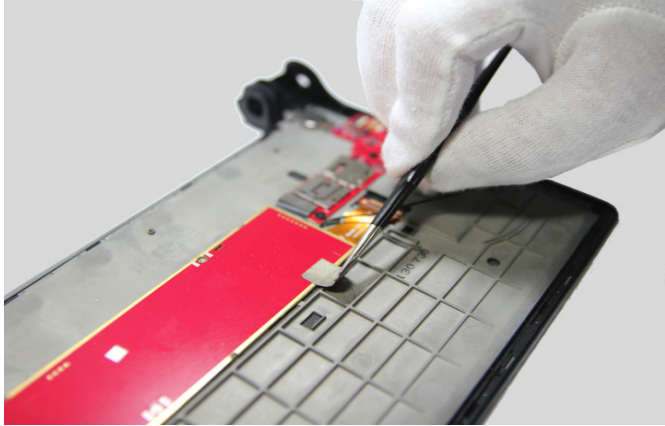
Figure 8-2 Removing the conductive fiber
