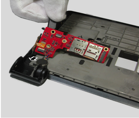
Figure 9-3 Detaching the vibrator motor
