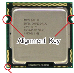
Yellow triangle is the Pin 1 indicator
