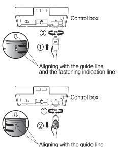
Aligning with the guide line and the loosening indication line
