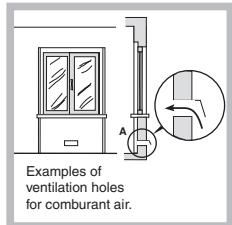
The air circulation system may take air directly from the outside by means of a pipe with an inner cross section of at least  $100 \text{ cm}^2$ ; the opening must not be vulnerable to any type of blockages.
