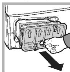
Release the three catches by turning 90° counter-clockwise then pull on the grip and remove from the dryer.
