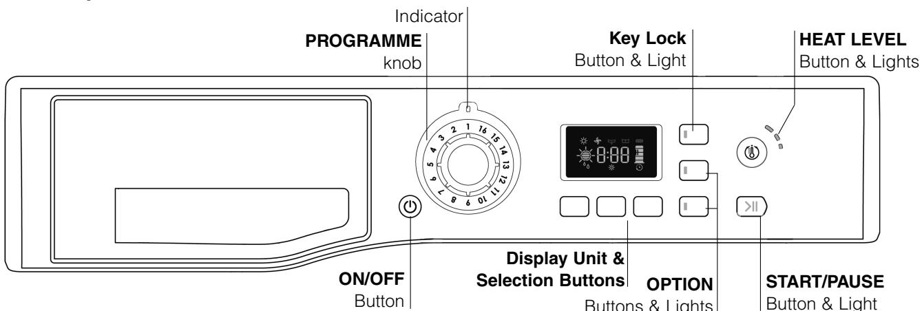
The **ON/OFF** button
