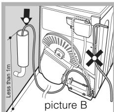
Then fit a suitable length of hose to position shown in picture B.
