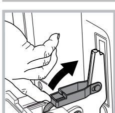
5. Rotate the pull-out hooks upwards until they touch the front of the oven.
