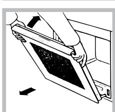
4. Holding the door by its two outer sides, slowly close it but not completely. Pull the door to remove it from its seat (see figure). To re-assemble the door follow the procedure in reverse order.
