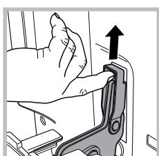
2. Lift the pull-out hooks located on the two hinges. If you cannot lift them manually, use a tool as a lever.
