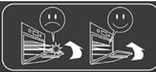
Make sure that the racks and dripping pans have been inserted fully before closing the door
