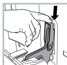
6. Push the pull-out hooks downwards, making sure they are steady and do not rotate forward.
