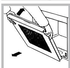
3. Grip the door on the two outer sides and close it approximately half way. Pull the door towards you, lifting it out of its slot (see diagram). To replace the door, reverse this sequence.
