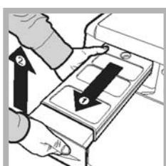
Pull the container out of the dryer and empty it into a sink or other suitable drain. Replace the water container securely.
