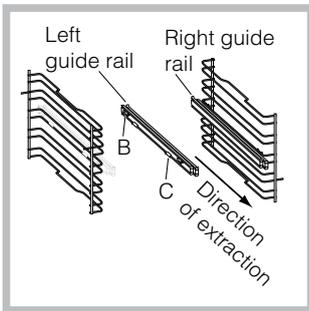
2. Choose which shelf to use with the sliding rack. Paying attention to the direction in which the sliding rack is to be extracted, position joint B and then joint C on the frame.
