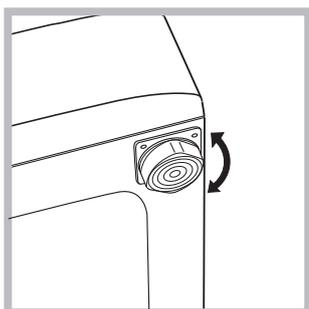
2. If the floor is not perfectly level, compensate for any unevenness by tightening or loosening the adjustable front feet (see figure); the angle of inclination, measured in relation to the worktop, must not exceed 2°.
