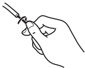
1: Strip the cover and twist the strands
