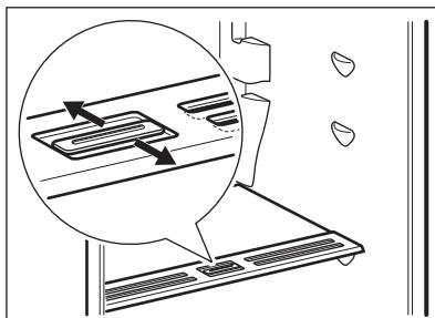
The glass shelf incorporates a device with slits (adjustable by means of a sliding lever), which makes it possible to regulate the temperature in the vegetable drawer(s).
