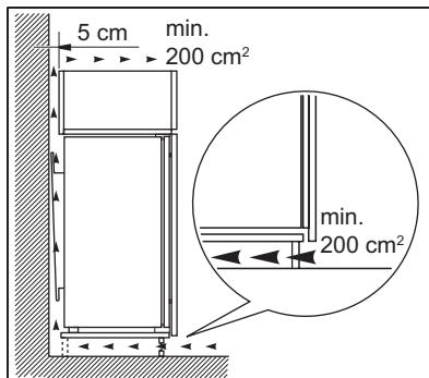
The airflow behind the appliance must be sufficient.
