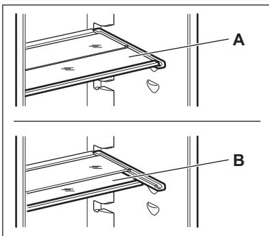
The walls of the refrigerator are equipped with a series of supports so that the shelves can be positioned as desired. For better use of space, the front half-shelves can be placed under the rear ones.
