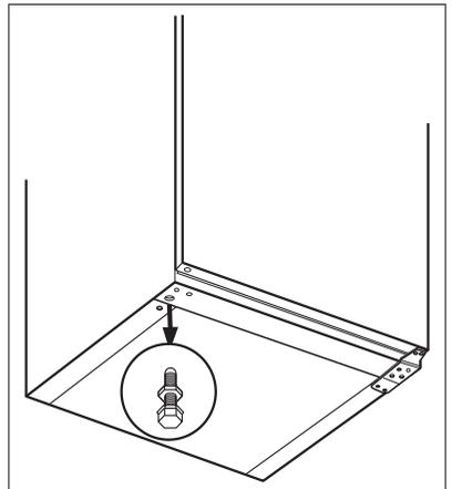
5. Unscrew the screws of the door bottom hinge. Remove the hinge. Put over the pin in the direction of the arrow.
