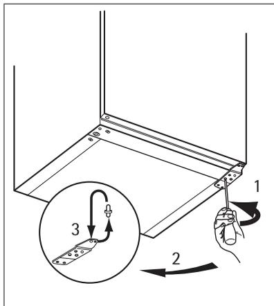
6. Unscrew and install the screw on the opposite side.
