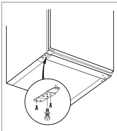
10. Remove the hinge. Put over the pin in the direction of the arrow. Install the hinge on the opposite side.
