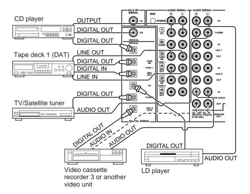
**NOTE:** All digital audio signal input jacks are applicable to the sampling frequency of 32 kHz, 44.1 kHz and 48 kHz.
