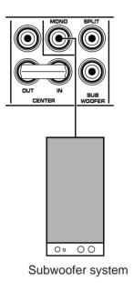
If you wish to obtain more presence in your listening room, the use of two subwoofers is recommended. To connect two subwoofers to this unit, connect the "left" SPLIT SUBWOOFER jack to the INPUT jack of the amplifier driving the left subwoofer, and the "right" SPLIT SUBWOOFER jack to the INPUT jack of the amplifier driving the right subwoofer, and then connect each subwoofer to the corresponding amplifier.
