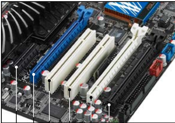
Slot PCI Express x4_1 Slot PCI 2.0 x16_1 (bleu, @x16 max.) Slot PCI 1 Slot PCI 2 Slot PCIe 2.0 x16_2 (blanc, @x16 max.) Slot PCIe 2.0 x16_3 (noir, @x8 max.)
