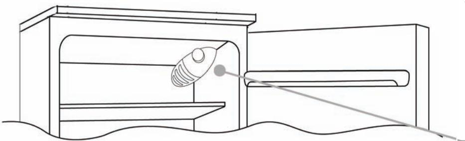
The thermostat box to control the appliance is located inside the fridge compartment on the top right. To check whether the appliance is functioning, make sure that the thermostat knob is not set on **0**.
