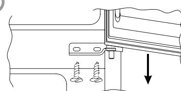
Retire as tampas (A) e (B), desaperte os parafusos e remova parcialmente o painel.
