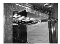
Place the grill reflector in the oven upper the grill heat element.
