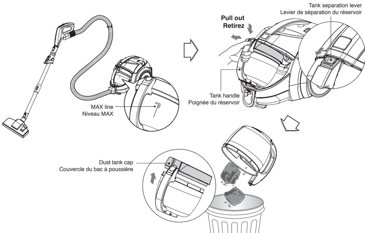
The dust tank needs emptying when the dust tank level reaches the MAX line.
