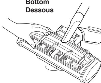
Since the vibrator inside is composed of precision parts, never disassemble the body.
