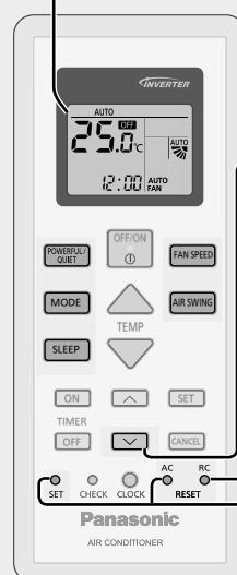
Press and hold for approximately 10 seconds to show temperature setting in °C or °F.
