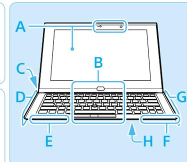
**G** USB port x 2 (Compliant with the USB 3.0 standard. The port with the lightning mark supports USB charging.)
