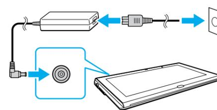
Plug the power cord and the AC adapter into an AC outlet and the computer.
