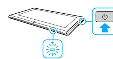
Press and hold down the power button until the power indicator light turns on.
