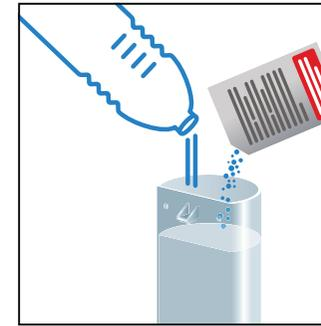
3. Fill the water tank with 0.5 L of fresh drinking water and add 1 *Nespresso* descaling liquid sachet.
