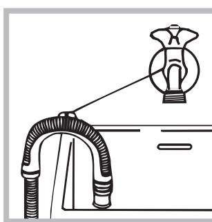
alternatively, place it over the edge of a basin, sink or tub, fastening the duct supplied to the tap (see figure). The free end of the hose should not be underwater.
