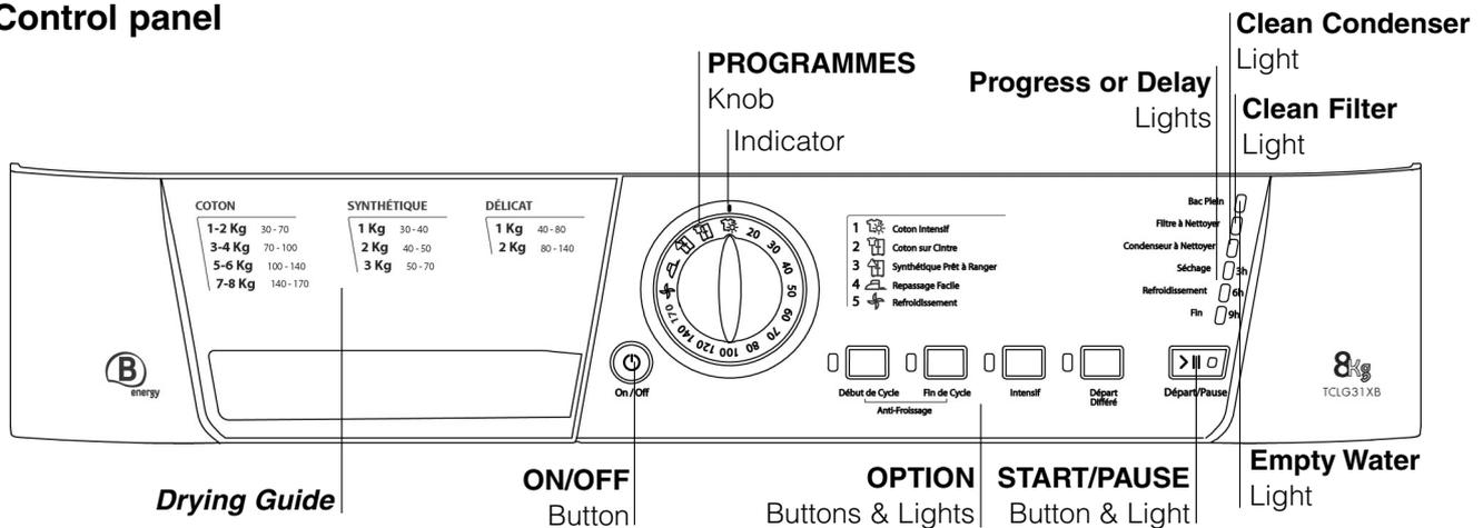
The **ON/OFF** button
