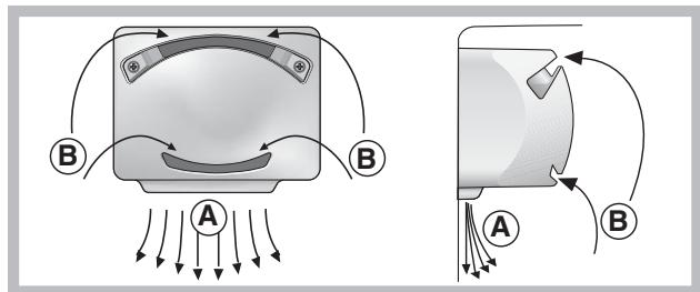
Pure Wind Plus maximises air circulation, improving the efficiency of the evaporator and helping to achieve the optimal temperature inside the refrigerator as quickly as possible each time it has been opened. The blown air (A) is cooled when it comes into contact with the cold wall, whereas the hotter air (B) is sucked up (see diagram).
