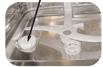
Filling with salt is essential to obtain a **good wash with no streaks**. The salt regenerates the resins, which soften the water by removing its limestone content unless the water is already sufficiently soft (see "Adjusting the water softener").
