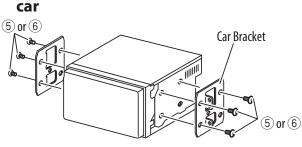
Select the appropriate type of screw for the mounting bracket: flat head (5) or round head (6).
