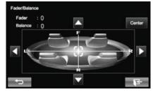
Fader: Adjust the front and rear speaker output balance.
