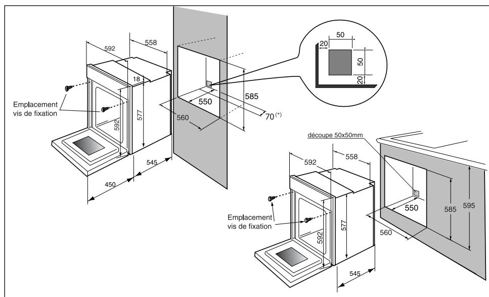
**The oven may be housed either under a work surface or built into a column that is open\* or closed with a suitable opening.**
